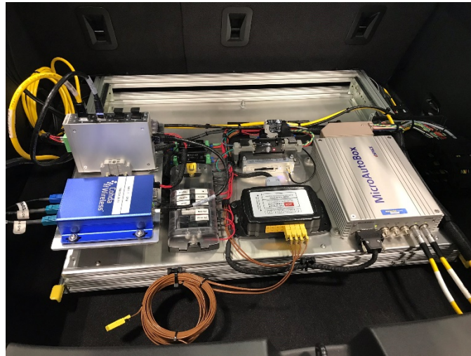
Figure 4-23: MTU Chevrolet Volt In-Vehicle Instrumentation Package.
